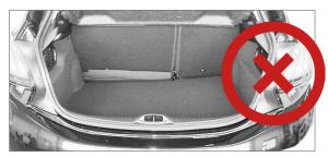
High threshold makes forklift loading impossible
